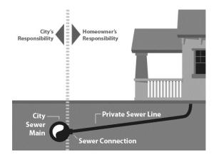
Waste travels from your home's plumbing system through the lateral to the municipal sewer main. Waste then travels through the municipal sewer lines to a wastewater treatment facility where the waste is properly managed.
